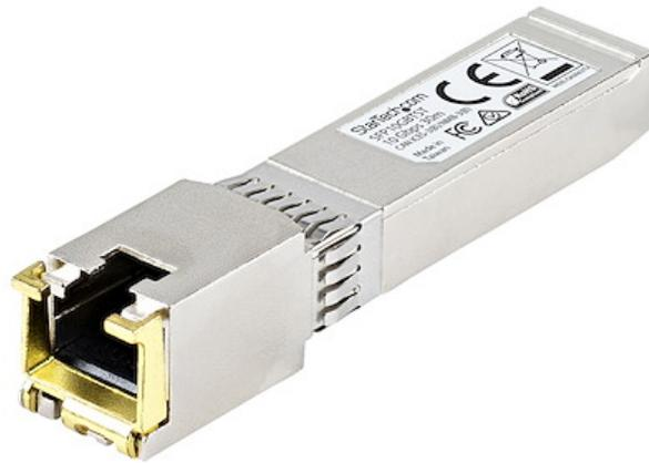
The SFP10GBTST is an MSA compliant copper SFP transceiver that's designed, programmed and tested to work with 10GBASE-T compatible switchess and routers. The SFP+ transceiver module supports a maximum distance of up to 30 m (98.4 ft.) and delivers dependable 10 GbE connectivity over copper cabling, which is a cost-effective alternative to fiber-optic cable setups. **Technical Specifications:**
