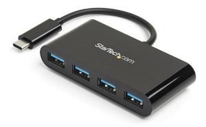
Here's a must-have accessory if you have a USB-C equipped computer but need more USB-A ports. This portable USB 3.2 Gen 1 hub expands your laptop or desktop connectivity by adding four USB Type-A ports through a single USB Type-C or Thunderbolt 3 port. And, because it's USB bus-powered, you don't need to connect an external power adapter, which makes travel more convenient and workstations less cluttered.
